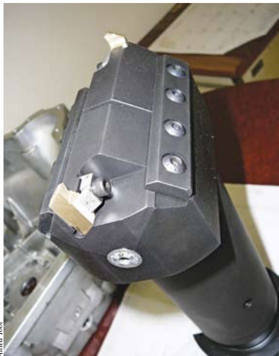
Two coated carbide inserts and a long, custom tool body are components of a special, adjustable hollow mill that allows Pioneer Products to decrease cycle time 20 percent for a job compared with the endmill and chamfering tool previously applied.
